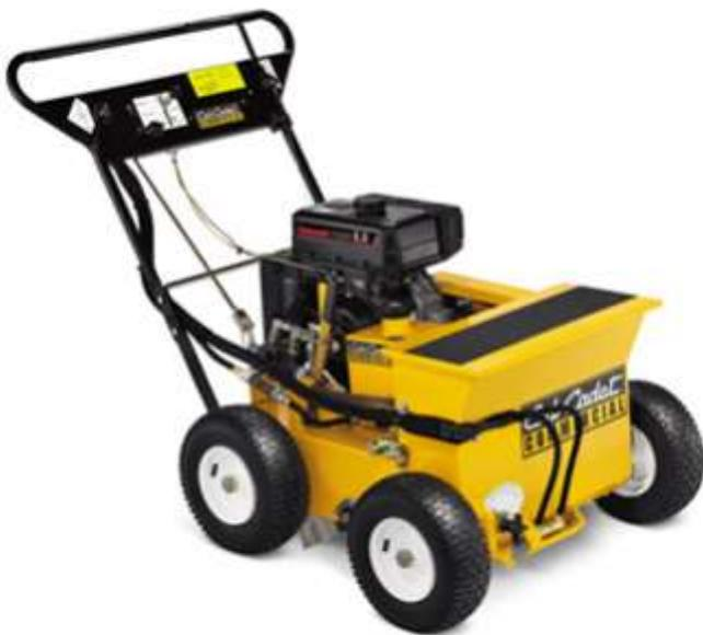
We have a fast, effective and affordable way to keep your problem turf areas lush. This machine, called a turf renovator, uses tines much like a power rake to cut slices in the soil and drop in grass seed. We use a mix of seed including a fast germinating variety for quick cover, blue grass, and shade tolerant grasses. The varieties most appropriate for the area then germinate and thrive. No additional irrigation is necessary.
